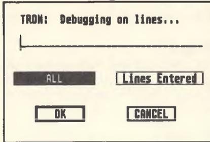
The Tron option displays the program's line number in the Command Window as each program line is executed.
