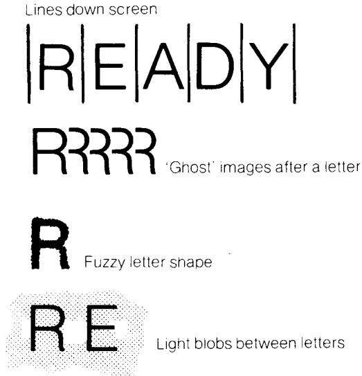
Fig. 1.6. Picture defects caused by faulty tuning.
