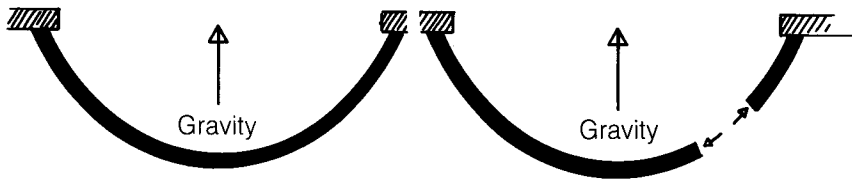
Figure 15.6 Tensile Forces Become Compressive Forces
