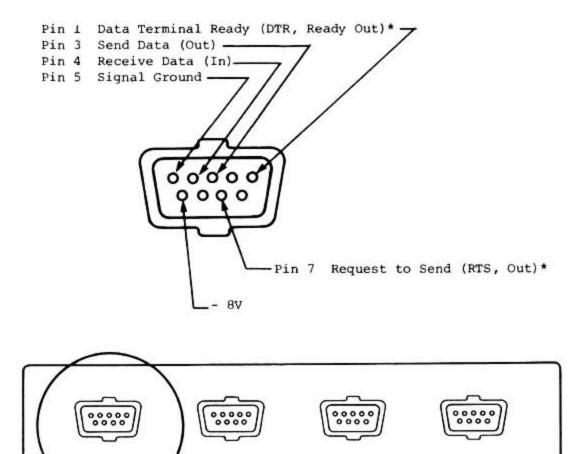
Figure 3. Pin functions of Serial Port No. 4 in 850<sup>TM</sup> Interface Module (9-pin female connector)
