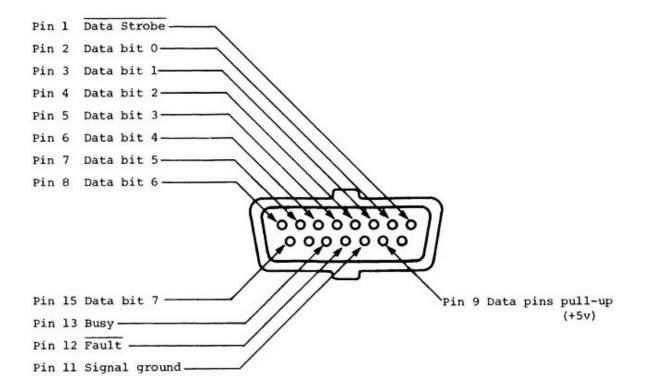
Figure 5. Pin functions of the Printer Port of the 850<sup>TM</sup> Interface Module (15-pin female connector
