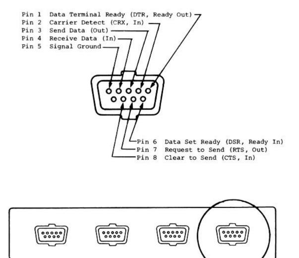
Figure 1. Pin functions of Serial Port No. 1 in 850<sup>TM</sup> Interface Module (9-pin female connector)
