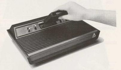
Always turn the console POWER switch OFF when inserting or removing an ATARI Game Program cartridge. This will protect the electronic components and prolong the life of your ATARI Video Computer System game.
