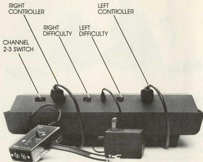
**Note:** Using any AC Power Adapter other than that designed for this ATARI 2600 Video Computer System can damage the unit.
