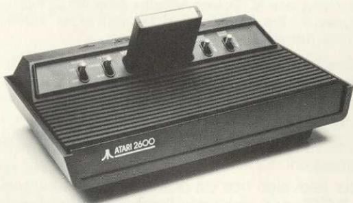
When removing the ATARI Game Program cartridge, pull it straight out of the console. Check to see that the POWER switch is OFF.
