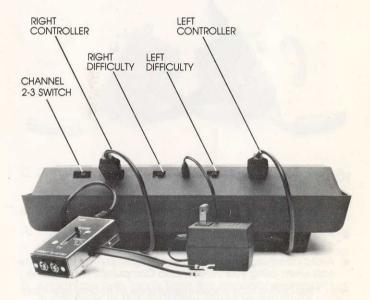
Note: Using any AC Power Adapter other than an ATARI CX261 Power Adapter can damage your ATARI 2600 Video Computer System.
