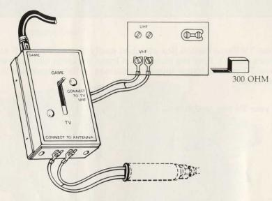
A. Move the "U" shaped slider to make connection between the two screws.
