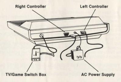
Attach the controllers by plugging them into the terminals on the back of the console. The controller jacks are designed to fit only one way, so do not try to force them into the terminals.
