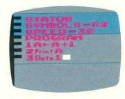
Notice that the STATUS region shows we have 52 "bytes" or symbols of memory remaining. The SPEED is set at 30 (SPEED = 30). Put the cursor into the white mode and depress the SLOWER key. Notice that every time you depress this key the speed decreases. Depress the FASTER key and the SPEED will increase.
