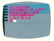
The cursor is directly to the right of the 2 in line 2. Now input **PRINT** using the green mode. Then, with the blue mode, input A and go to a New Line. Your display will look like this:
