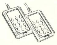
To connect the two controllers, slide the tongue of the left controller into the groove on the right controller. The two Keyboard Controllers, locked together, form a 24-key Keyboard used to enter your program and to control the display on your television screen.
