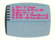
In this program we have given two **IF/THEN** commands. If the conditions set up in the first command are not met (line 4) the computer will move to the next line (line 5). Given enough memory, there can be several commands between any two **IF/THEN** commands.
