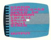
Press the RUN/HALT key and start the program. In line 2, the computer is instructed to PRINT A. When it reaches this command, it will print the current value of A in the OUTPUT region. Watch the SYMBOLS area of the STATUS region.
