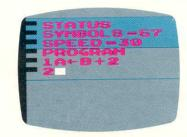
If you make an error in entering your program, it can be erased using the **ERASE** key. Notice that the **ERASE** key is **not** color coded. It can be used when the shift key is in any color mode.
