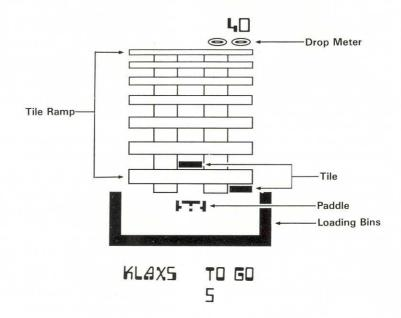
**Paddle** moves from side to side in the paddle slide and catches tiles, flips them into the bins or back up the ramps.
