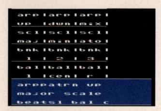
Pressing the Game Select switch will activate the Advanced Options Mode. Here, you can set the arpeggiator pattern (arp up, dwn, mix), change the scale setting (scl), set the current beat bank (bnk), and change the balance setting.
