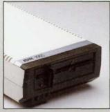
5 Insert a diskette carefully into the drive opening with the label facing up and toward you. After sliding the diskette all the way into the slot, turn the latch on the front of the drive to the down (vertical) position.
