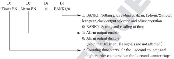
\*) When the Timer EN is set to 0, the 1-second counter and higher-order counters than the 1-second counter stop. If any carrying occurs in the lowerorder counters than the 1-second counter while the Timer EN is 0, carrying will be held and avoided until the Timer EN changes from 0 to 1. Thus, no apparent delay is produced when the duration of the Timer EN = 0 is less than one second.
