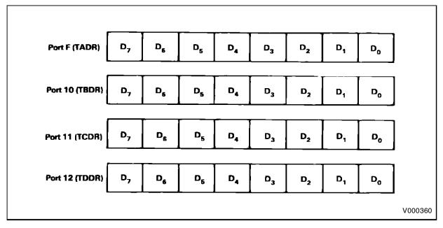
Figure 13 : Timer Data Registers (A, B, C, and D).
