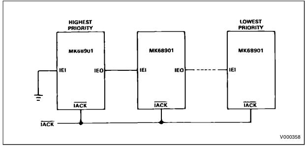
Each interrupt channel responds with a discrete 8bit vector when acknowledged. The upper four bits of the vector are set by writing the upper four bits of the VR. The four low order bits (bit 3-bit 0) are generated by the interrupting channel.
