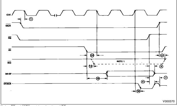
**Note** :  $\overline{\text{CS}}$  and  $\overline{\text{IACK}}$  must be a function of  $\overline{\text{DS}}$ .
