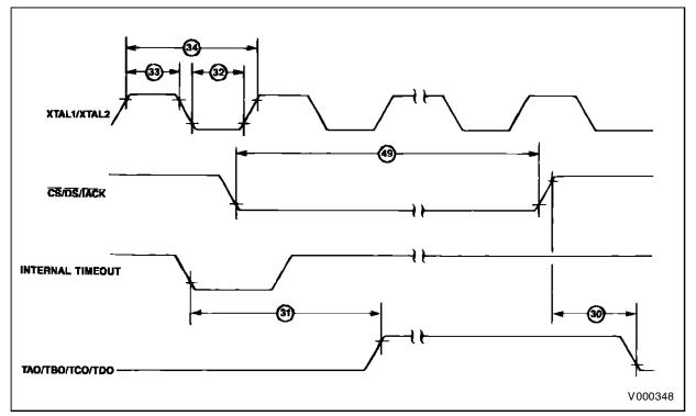
Figure 30 : Reset Timing.
