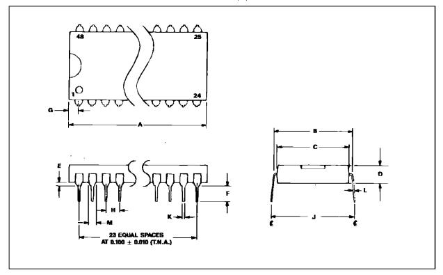
MK68901 48-PIN PLASTIC DUAL-IN-LINE PACKAGE (N)
