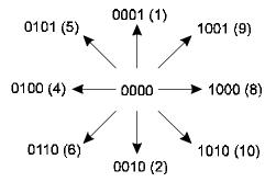
Joysticks may be interrogated at any time by sending an interrogate command (as described later in this chapter). The packet response to this command is 0xFD followed by the **BYTE** report of joystick 0 and 1 (as shown above).
