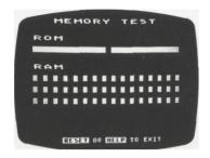
During the RAM test, 48 squares—each representing a RAM sectionare tested. The remaining 16K RAM is available only with certain software programs. If a square turns white, then green, the corresponding section is good. If no square turns red, the RAM is okay.
