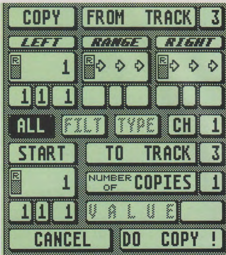
The Multi-Toolbox is used to copy, move or delete tracks or any defined events.
