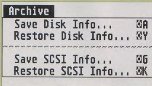
The Save Disk Info option saves partition information which includes the boot sector, FAT and Directory sectors. Save SCSI Info saves sector 0 which contains essential information on the disk's structure.
