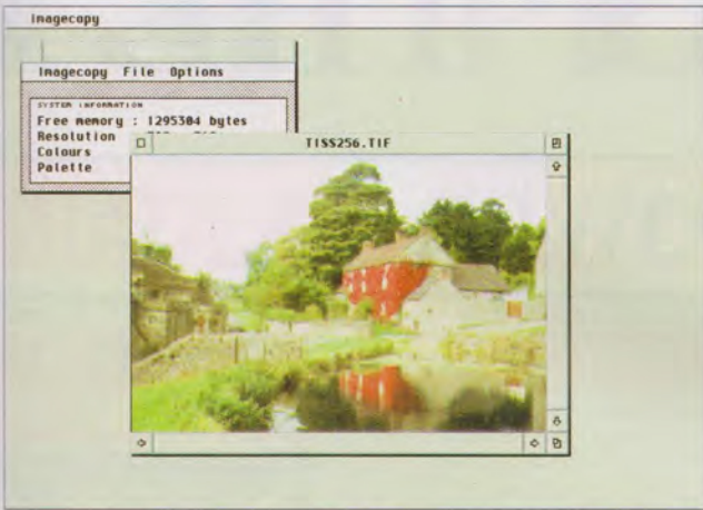
The main advantage of an RGB monitor is the ability to use interlace to display True Colour modes with overscan. This snapshot was taken at a resolution of 768 by 480 dots.
