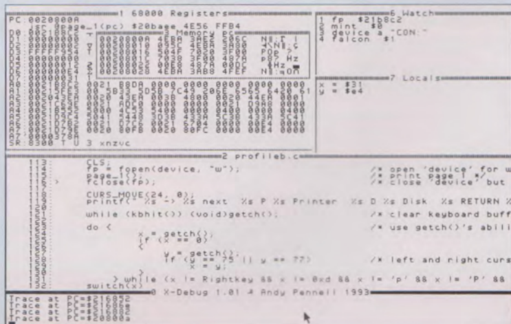
Single-stepping through source code in Window 2 with some globals shown in Window 6 and locals in Window 7. The memory dump in Window 3 is locked on to the PC register. The Register Window and Command Window are also shown.
