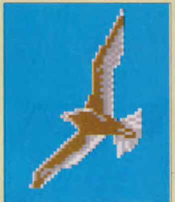
Part of a Degas picture showing a good example of anti-aliasing with a medium grey being used to break up the edges of the seabird's wings.
