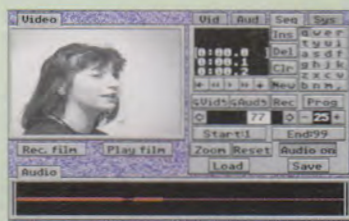
Sequences can be set up to play any film or sample whenever a certain key is pressed.
