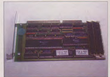
Face to face - the Janus board with its 16MHz 68000, TOS 2.06 ROMs and on-board SIMMs.
