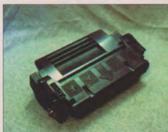
Most modern printers use a disposable cartridge holding both toner and the drum.
