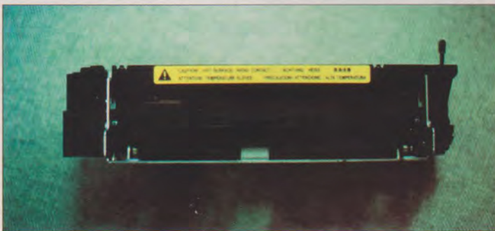
A typical fuser assembly showing the pair of rollers – damage this and you're likely to receive a £300+ bill!
