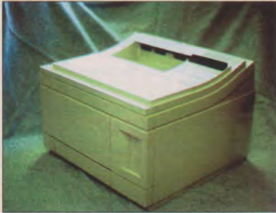
Hewlett Packard's LaserJet 4 uses a charge transfer roller to avoid ozone creation.
